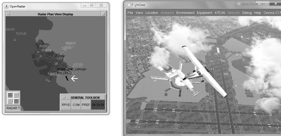
**Fig. 4.** Flight Gear simulator connected to modified OpenRADAR. Multiple black dots next to the white arrow in the left part of image represent the history of plane movements on virtual radar screen with KSFO airport overlay
